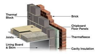
Fit the insulation layers between the joists ensuring all joints are close-butted to avoid air gaps. Overlap additional layers to reduce thermal bridging and air gaps.
